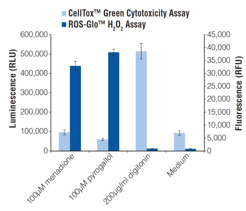
This multiplex allows determination of ROS production and cytotoxicity. It also allows total cell number analysis for normalization.
