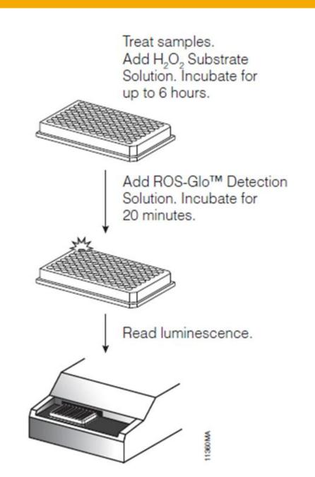
The ROS-Glo™ H<sub>2</sub>O<sub>2</sub> Substrate is added to the wells of cultured cells with test compounds.
