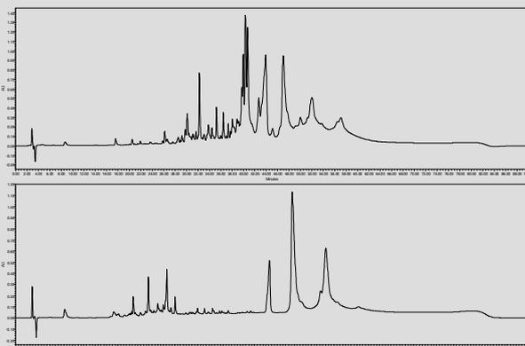
RP-HPLC chromatograms for batch and microfluidic experiments after 30 seconds reaction time (1µL.min<sup>-1</sup>)
